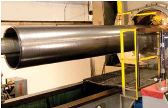
External Cold Roll Extruded cylinder typical starting blank, demonstrating material economy and axial growth in length while keeping the I.D. constant during External Cold Roll Extrusion.
