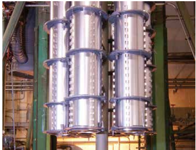
Patriot motorcase & nozzle Material: D6AC
