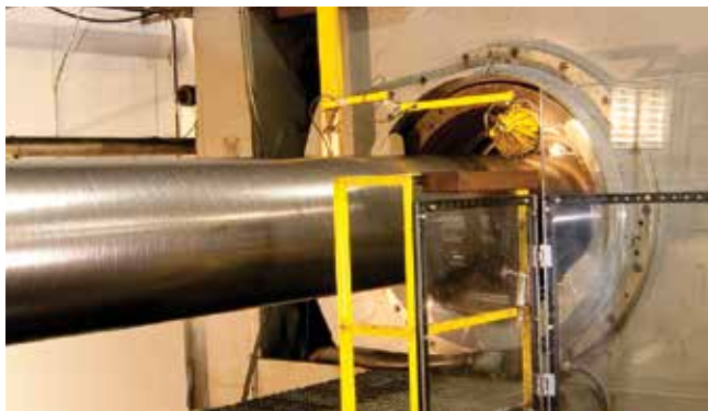
External Cold Roll Extruded cylinder typical starting blank, demonstrating material economy and axial growth in length while keeping the I.D. constant during External Cold Roll Extrusion.
