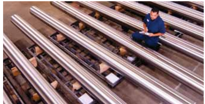
Internal Cold Roll Extruded cylinder typical starting blank, demonstrating material economy and axial growth in length while keeping the O.D. constant during Internal Cold Roll Extrusion.
